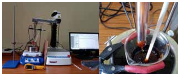
Fig. 7.5: Setup for determination of cohesion-adhesion behavior of seedlac samples
