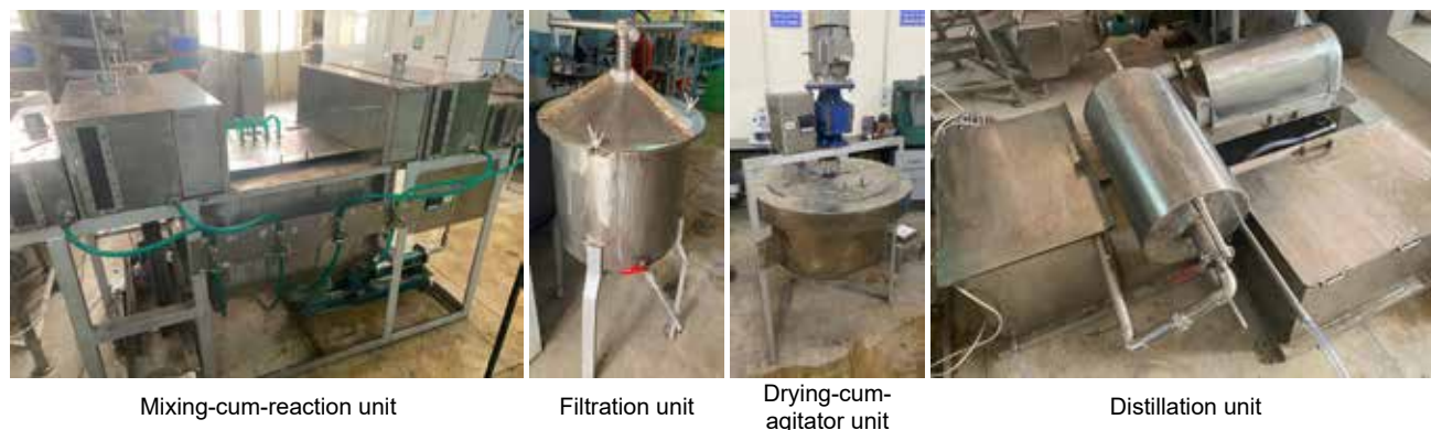
Fig. 7.1: View of fabricated units under guar gum derivative pilot plant
