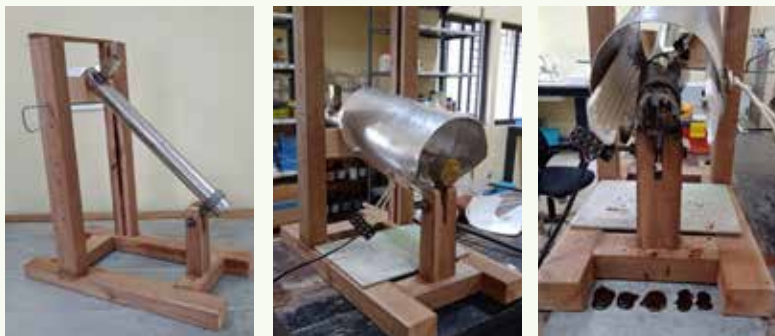
Fig. 3: Developed manually-operated ram-extruder prototype
